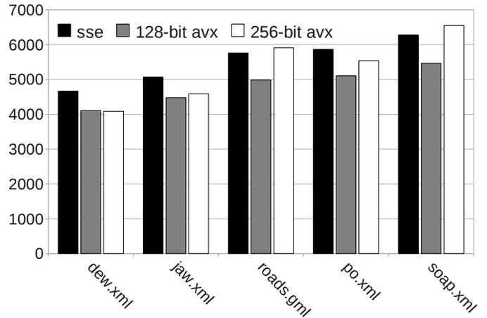
Figure 20: Parabix2 Performance (y-axis: CPU cycles per KB)
