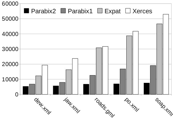
Figure 13: Processing Time on Core-i3 (y-axis: Total CPU Cycles per kB)
