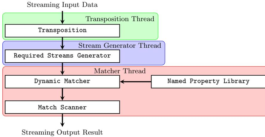
Fig. 4: Data flow in an icGrep execution
